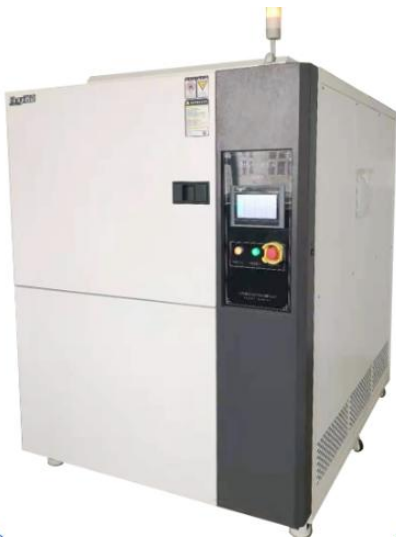
20 L constant temperature and humidity test chamber
