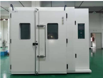
3.6 m3 constant temperature humidity laboratory
